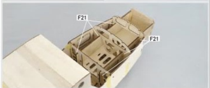
4.27 Insert engine box into fuselage. Apply epoxy glue to all surfaces in contact. Glue in F19, F20, F21 and F22A.
