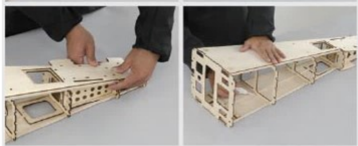
4.4 Glue in F9C, F10, F11 and F12, then glue in the right side panel. Make sure all the latches are fully inserted into corresponding slots.
