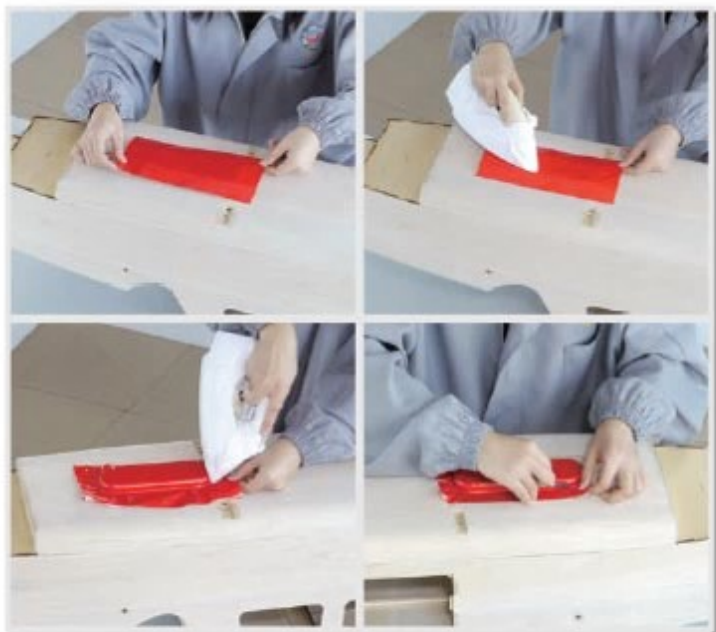
6.3 First work on bottom of fuselage. Cover landing gear block with covering then apply hot iron. Iron around the landing gear block until the covering conform to the shape of landing gear block. Allow 3 mm overlap and cut away excess covering material.
