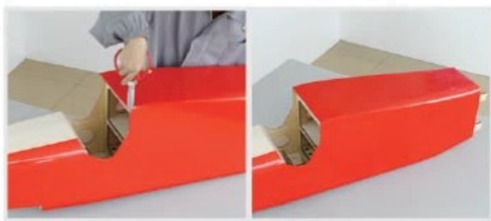
6.6 Iron on top fuselage covering, apply heat to make covering conform to corners.
