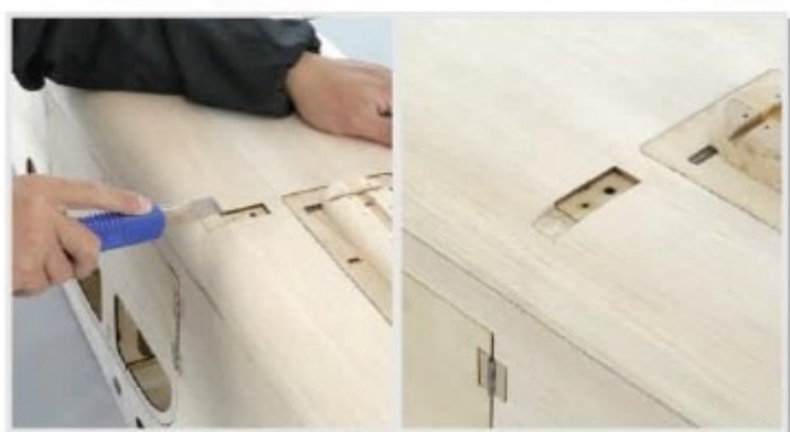
4.32 Cut out landing gear slot.
