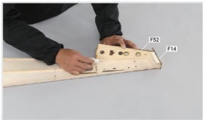
4.2 Glue in F14 and F52, make sure all the latches are inside corresponding slots.
