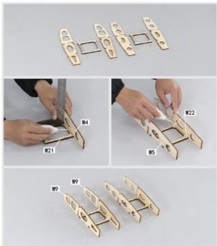
1.6 Glue W21 between W4 and W5, W21 between W9 and W9. Make sure the half rib is facing inward and join to W21. Glue W22 for reinforcement.
