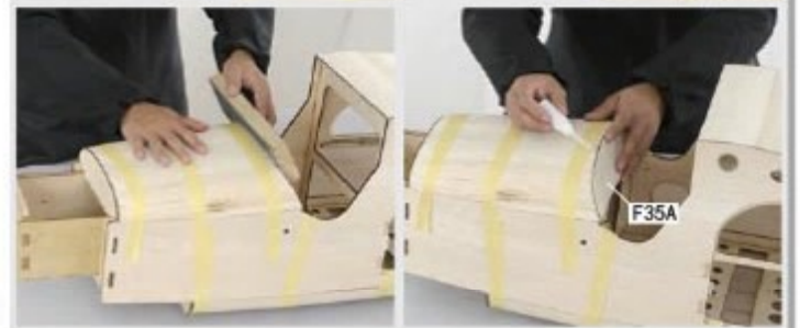
4.29 Apply slow curing glue to surfaces in contact with F24. Apply moisture to outer 6 cm portion of F24 then put on top of frame. Use tape to hold F24 in position. When cured remove rough surface by knife and sand paper. Glue in F35A.
