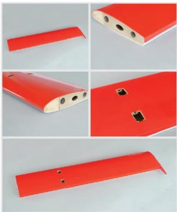
6.22 Cover top of wing. Allow 3 mm overlap at both ends and total 6 mm overlap at leading edge. Cut openings for wing tube latch hatch.
