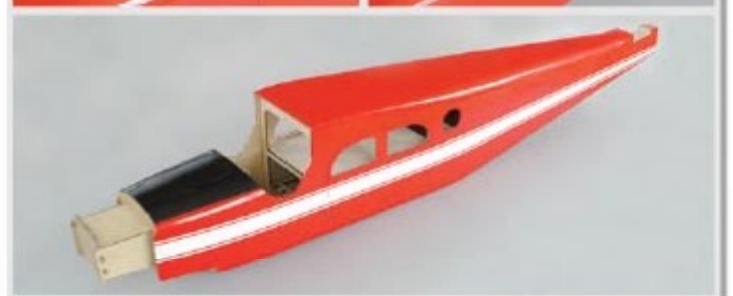
6.12 Install cowling and tail section to the fuselage. With reference to cowling trimming pattern, add on fuselage side panel trimming. After trimming is done, cut trimmings at junctions to free door and servo mount.
