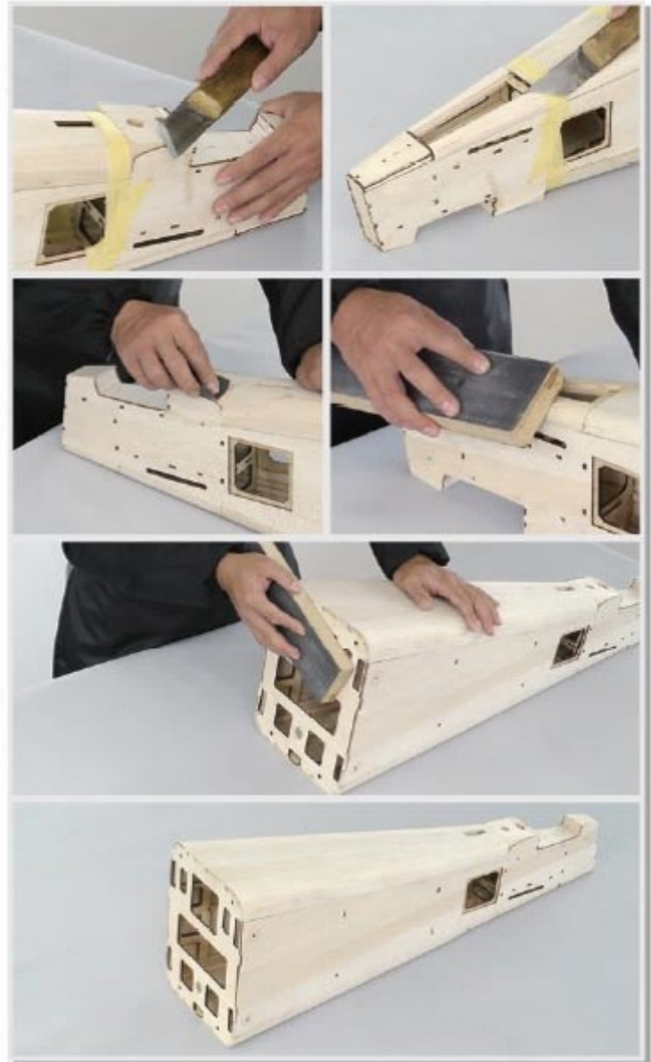
4.13 Remove rough edges with knife and sand paper.
