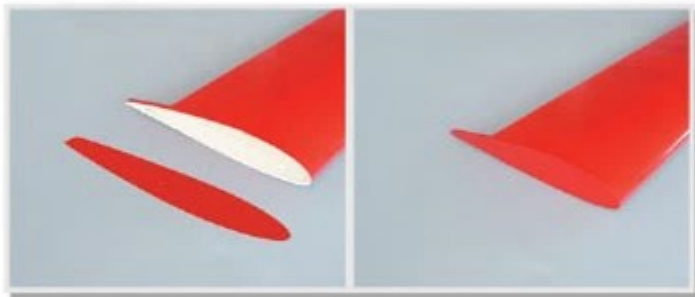
6.23 Cover wing tip. Allow 3 mm overlap.
