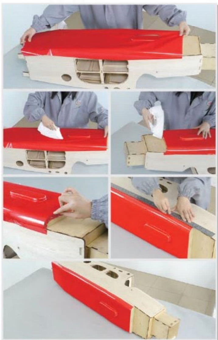
6.4 Lay bottom on fuselage. Align landing gear block hole and spread covering evenly on bottom of fuselage. Apply hot iron until covering stick and conform to balsa surface. Allow 3 mm overlap on ends and 20 mm on left and right side of fuselage. Trim away excess covering.
