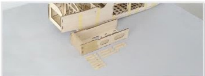
4.26 Glue in F5C, when cured glue in F26. Apply slow curing glue to surfaces in contact with F27. Apply moisture to outer 6 cm portion of F27 then put on top of frame. Use tape to keep F27 in position, more tape on curved section. When cured apply glue for reinforcement.
