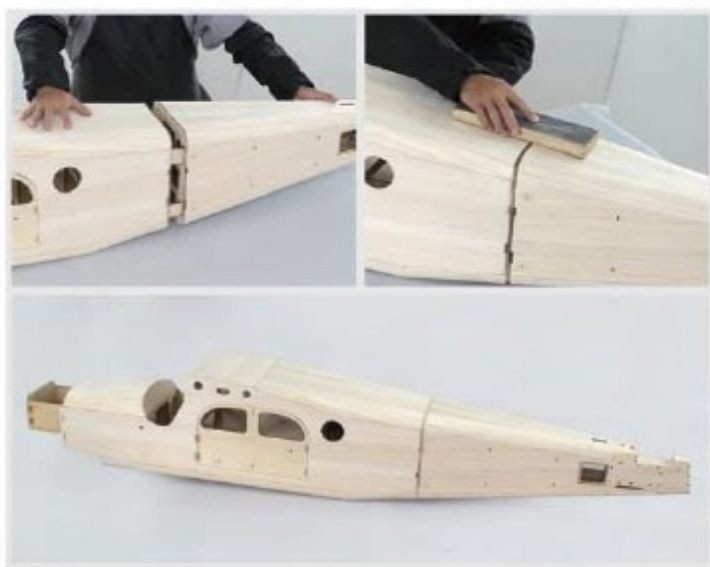
4.34 Trial fit tail section to front section and sand down joining area.
