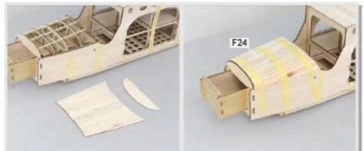
4.28 Glue in F2B and F3B. Glue in F33 and F34. Make sure tapered surface is facing outwards. Then glue in F35.
