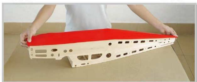
11.3 Place covering on fuselage bottom, completely covering the surface with 5mm overhang at all sides.
